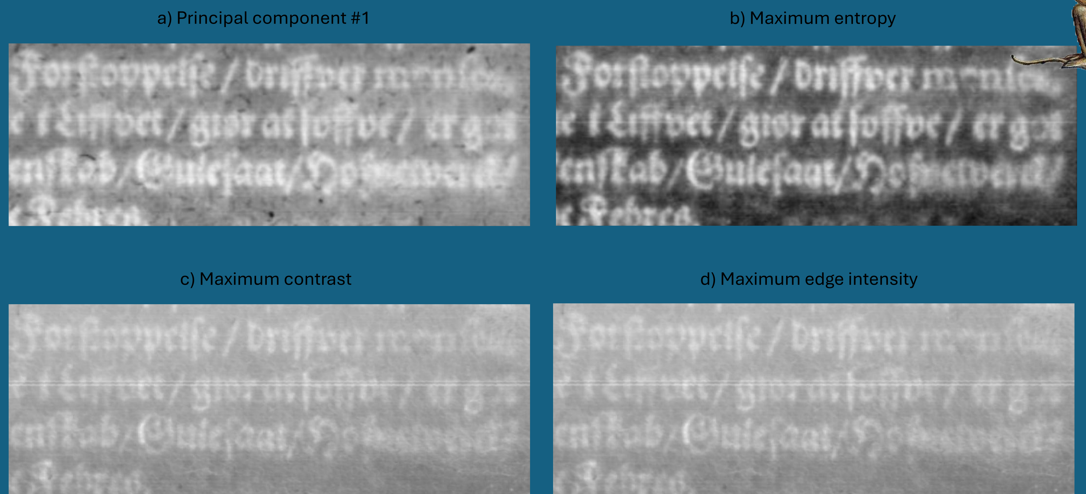
Fig. 4: Optimal principal component combination for maximum b) entropy, c) contrast, and d) edge intensity compared to a) the most readable principal component
